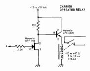
A negative voltage at point "A" (about -3. Ovolts or greater) will stop the F.E.T. conducting and allow the base voltage on the transistor to rise so that it will conduct thus operating the relay.
